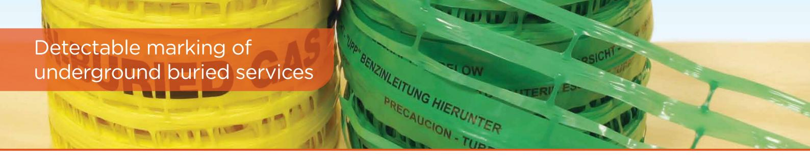
With a traceable stainless steel wire laminated between a printed underground warning tape and plastic mesh, underground services can be located using a CAT & Genny while providing a clearly visible warning of the danger below.
