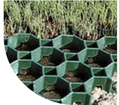
BODPAVE 40 porous grass pavers are an interlocking cellular paving grid system for grass and ground reinforcement applications where there is regular pedestrian or vehicle use. BODPAVE 40 permeable paving grids allow full rainwater penetration and are manufactured from UV stabilised 100% recycled HDPE, in black or green. BODPAVE 40 pavers are strong, chemically inert & non-toxic, enabling them to provide a durable, safe & sustainable eco-friendly surface for trafficked areas.
